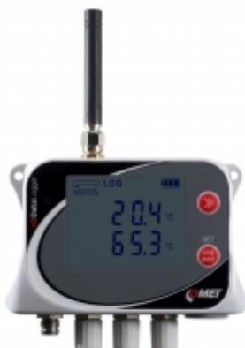
GSM Datalogger is designed to record temperature from four external Pt1000 probes. In case of exceeded set limits, SMS and JSON messages can be sent via GPRS data connection. Measured values can be sent to the internet storage [COMET Cloud](#), which is a complete monitoring, alarm and analysis system.
